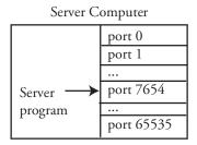
2. The client connects to the server on port 7654. It uses a local port that is assigned automatically, in this case, port 20314.
