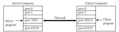
The server program can now communicate over a socket bound locally to port 7654 and remotely to the client's address at port 20314.
