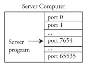
2. The client connects to the server on port 7654. It uses a local port that is assigned automatically, in this case, port 20314.
