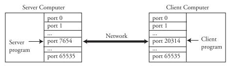
The server program can now communicate over a socket bound locally to port 7654 and remotely to the client's address at port 20314.
