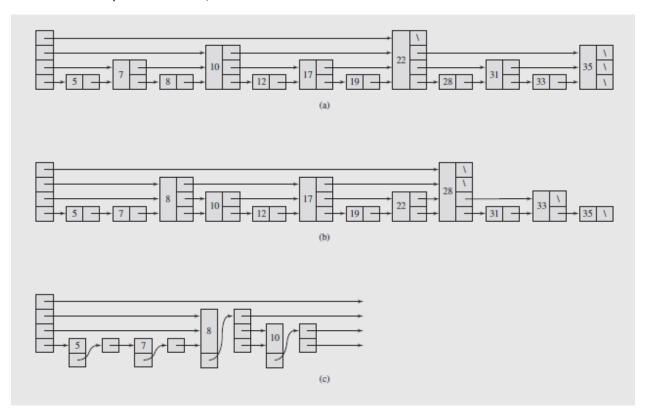
A skip list with (a) evenly and (b) unevenly spaced nodes of different levels; (c) the skip list with pointer nodes clearly shown
