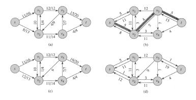
**Figure 26.3** (a) The flow network G and flow f of Figure 26.1(b). (b) The residual network  $G_f$  with augmenting path p shaded; its residual capacity is  $c_f(p) = c(v_2, v_3) = 4$ . (c) The flow in G that results from augmenting along path p by its residual capacity 4. (d) The residual network induced by the flow in (c).
